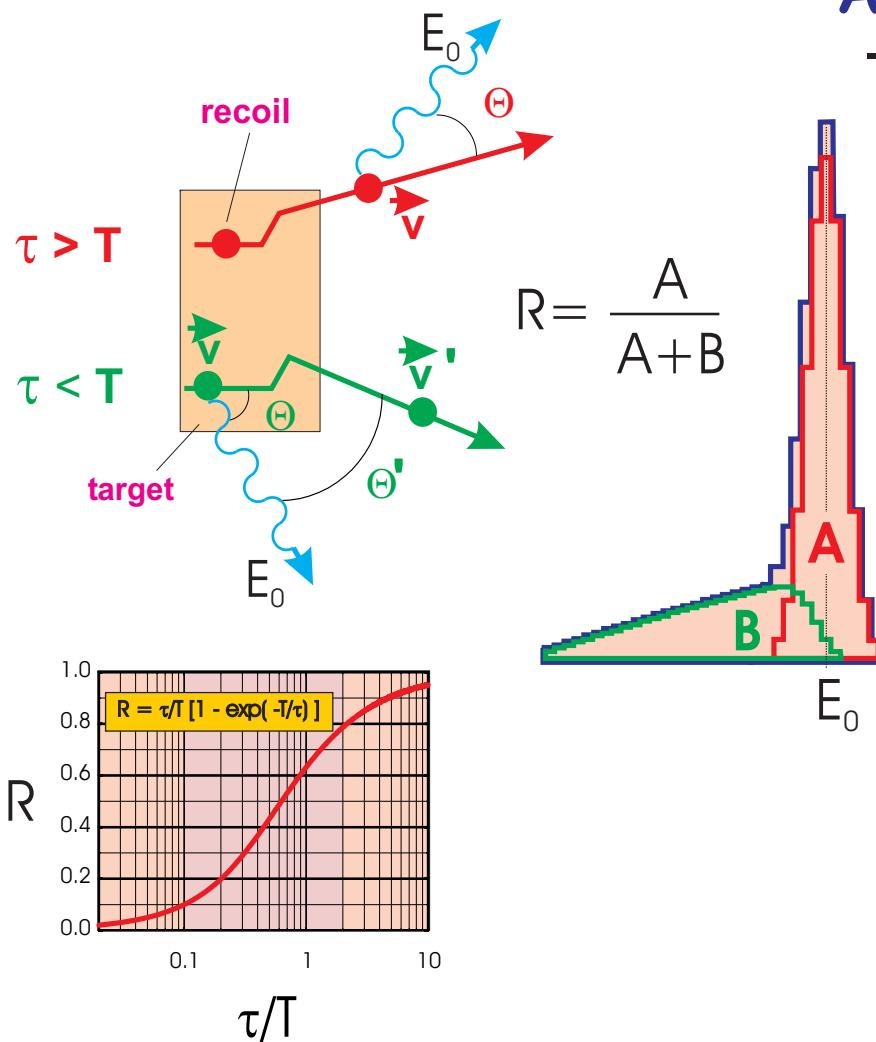
The range of measured lifetimes can be chosen by a selection of the target thickness.
