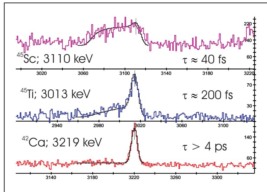
In the measurement  $\tau$  ranging from 40 to 800 fs could be determined.
