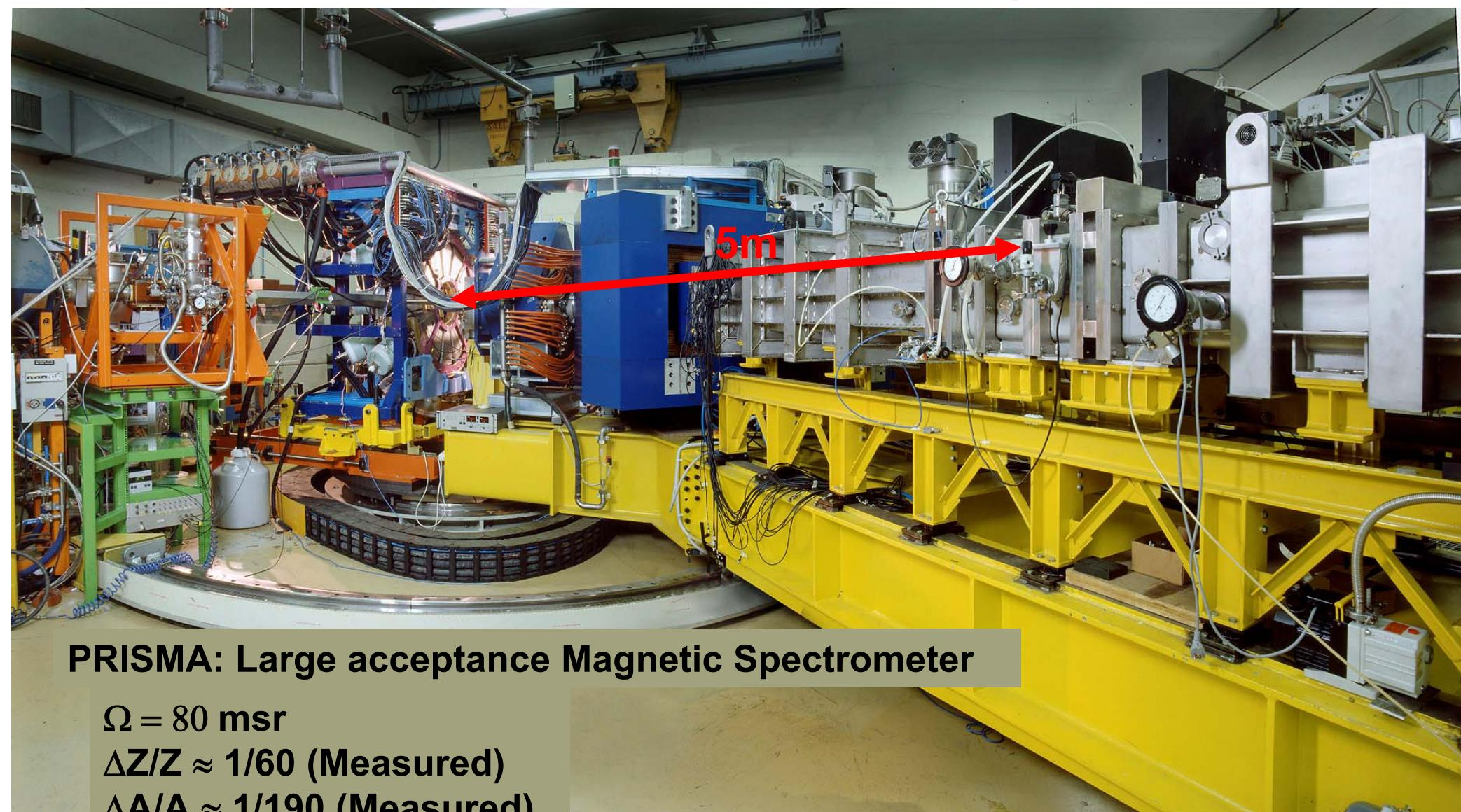
PRISMA: Large acceptance Magnetic Spectrometer
